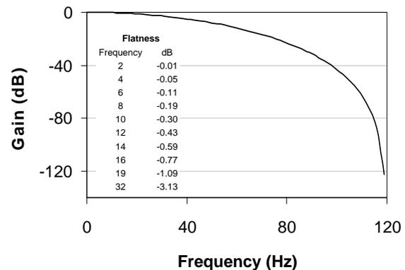
Figure 17. 120 Sps Filter Magnitude Plot to 120 Hz
