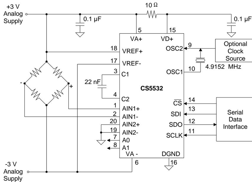
**Figure 23. CS5532 Configured with  $\pm 3$  V Analog Supplies**
