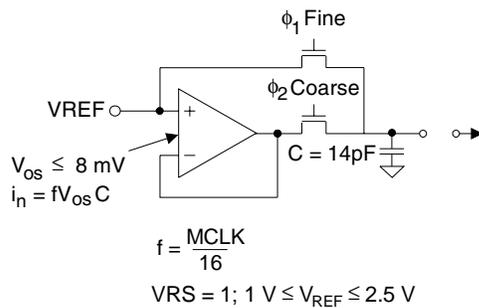
**Figure 9. Input Reference Model when VRS = 1**
