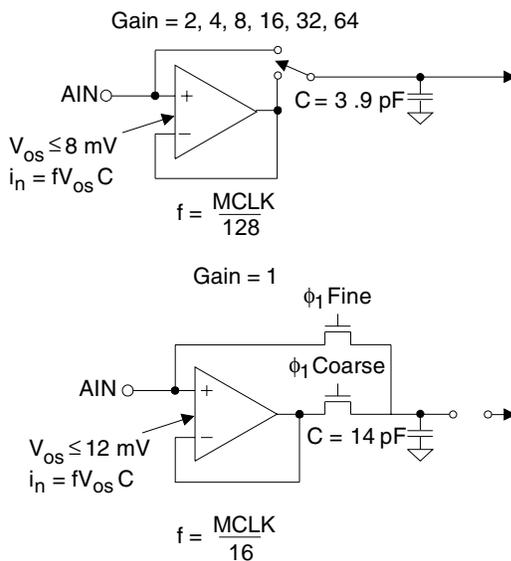
**Figure 4. Input models for AIN+ and AIN- pins**
