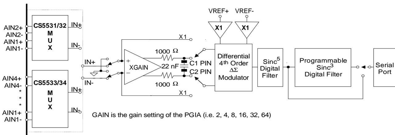
**Figure 3. Multiplexer Configuration**
