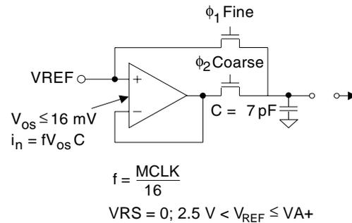
**Figure 10. Input Reference Model when VRS = 0**
