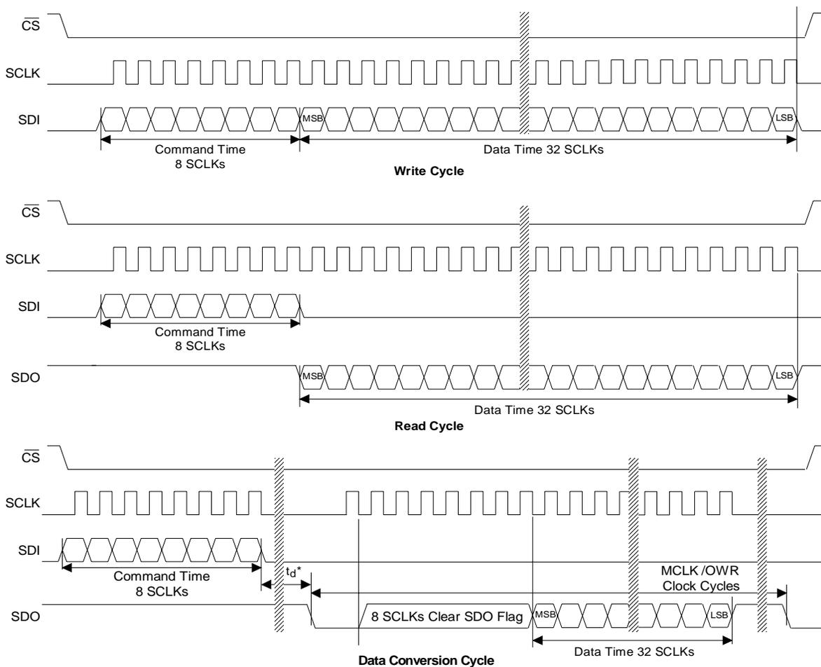
\*  $t_d$  is the time it takes the ADC to perform a conversion. See the Single Conversion and Continuous Conversion sections of the data sheet for more details about conversion timing.
