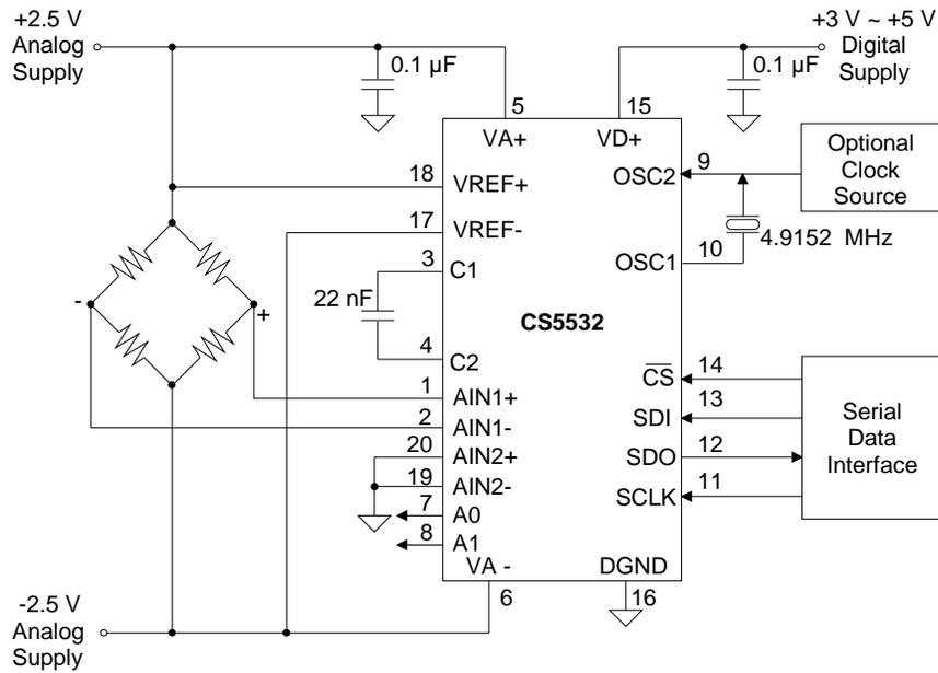
**Figure 22. CS5532 Configured with  $\pm 2.5$  V Analog Supplies**
