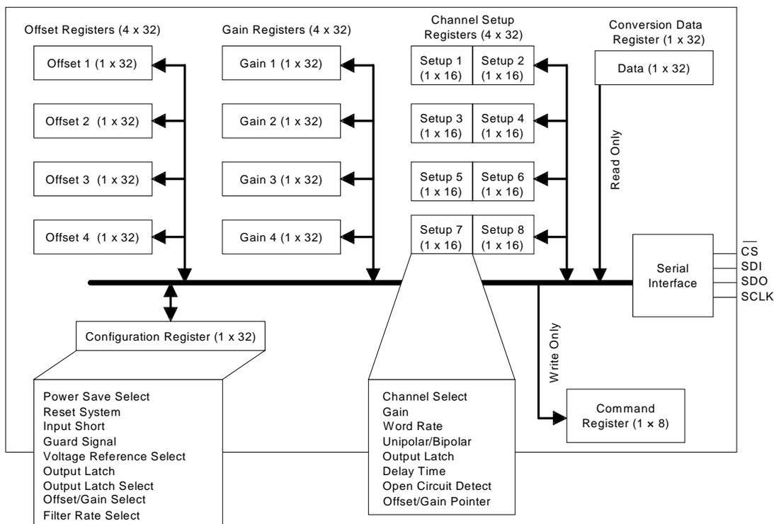
**Figure 6. CS5532/34 Register Diagram**
