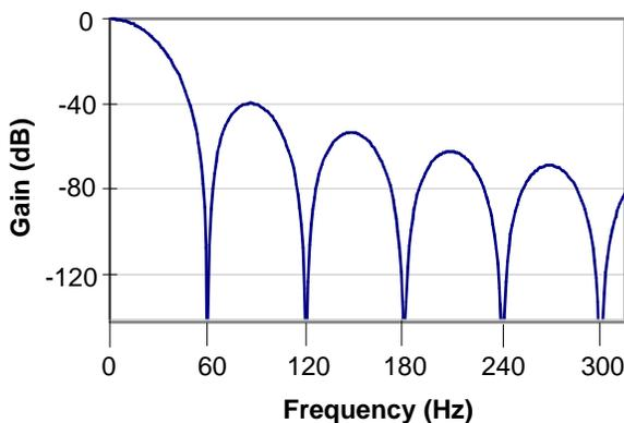
Figure 16. Digital Filter Response (WR = 60 Sps)
